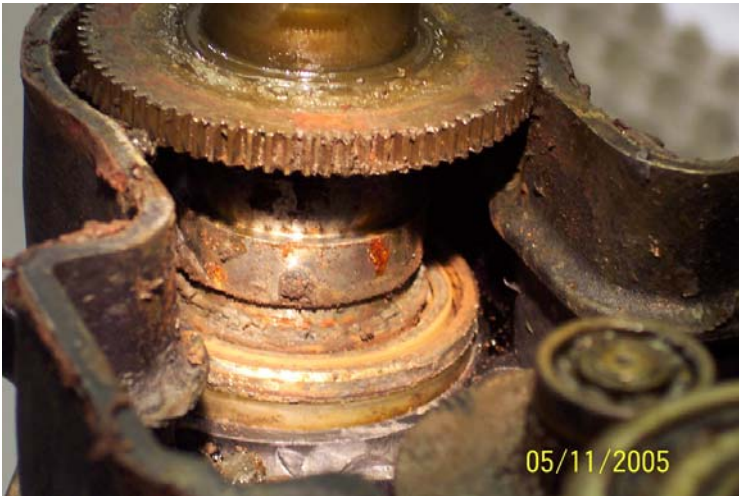
Close-up of one trim actuator's corroded internal parts
