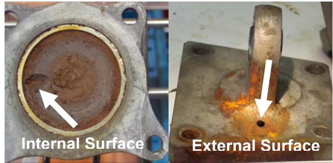
Note plugged drain hole at internal surface; external surface appears to be open.
